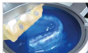
9. Lift the foil reception, loosen the foil securing ring and remove the foil together with the model pot through the foil reception. Loosen model and remove it.
